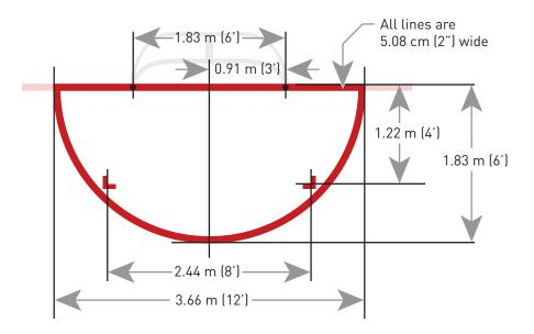
A semi-circle six feet 1.83m (6') in radius and two inches (5.08cm) (2") in width shall be drawn using the centre of the goal line as the centre point. In addition an "L"-shaped marking of five inches (12.7cm) (5") in length (both lines) at each front corner will be painted on the ice. The location of the "L"-shaped marking is measured by drawing an imaginary four foot (1.22m) (4') line from the goal line to the edge of the semi-circle.
